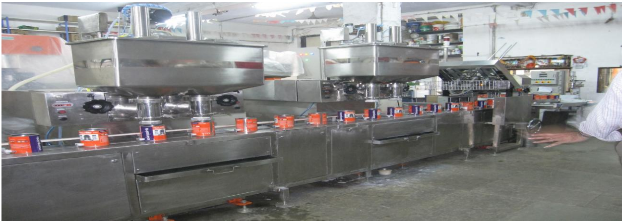
Fig 1.1 Paint filling Station
